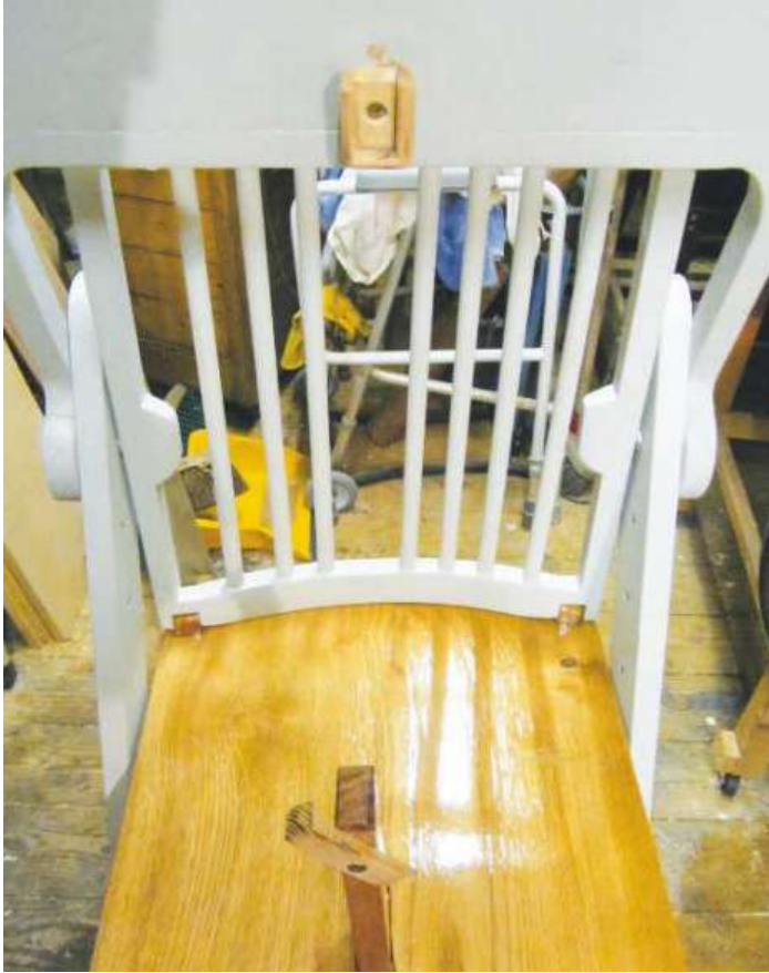
▲ Pic.8 A turnbuckle locks the tray's support post into place. The right-hand wall of the housing above extends enough to stop the turnbuckle swivelling too far
